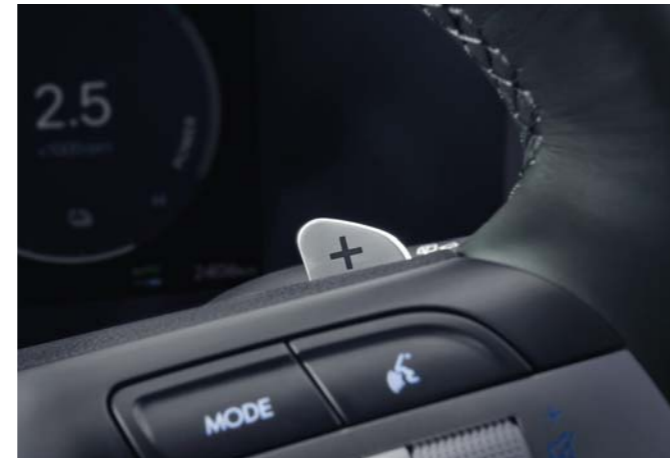
Hybrid Exclusive Features Paddle Shifter-Regenerative Braking Mode
