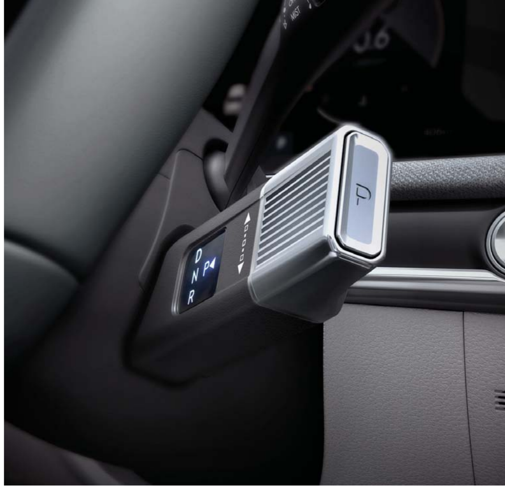
Column-type Shift by Wire (SBW)
